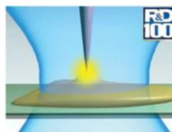
SPM-combined Raman spectroscopy system for single molecule experiments (in-plane resolution for spectroscopy is ~50 nm). Tip enhancement of Raman allows detecting signal from single molecule.
