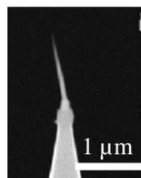
1 micron-long Whisker tip grown on silicon probe apex provides extremely high aspect ratio, tip radius is about 10 nm.
